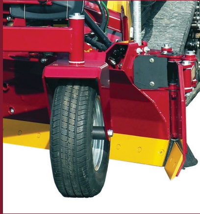
Hydraulic wings control material in both directions
