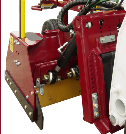
Rear blade to precision grade in reverse
