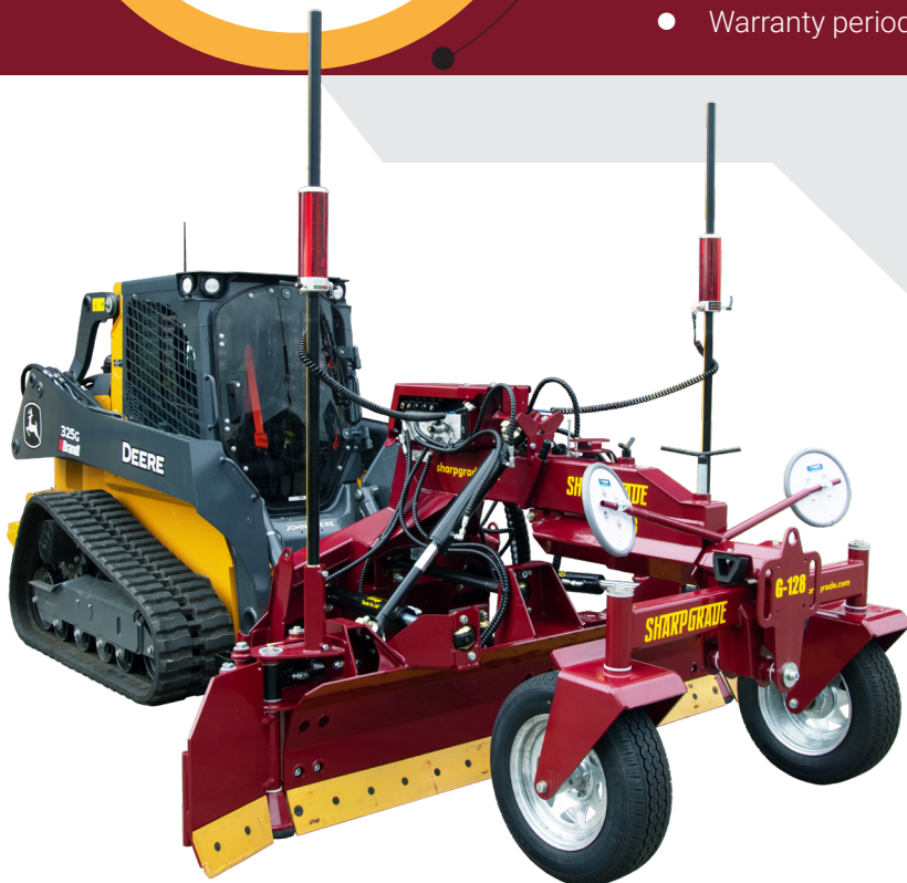
Robust hydraulic wings grade in either direction
