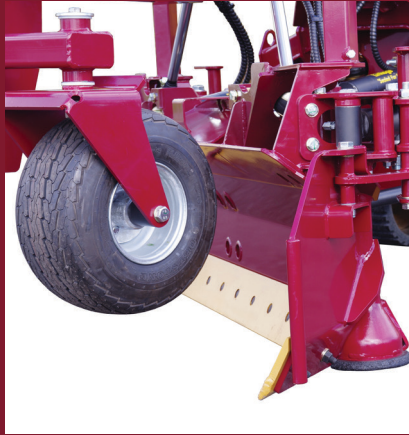
Hydraulic wings control material in both directions
